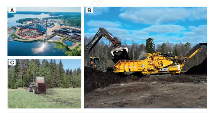
Figure 1. Production and utilisation stages of bark waste, a side stream of the UPM Plywood industry. Spruce (*Picea abies* (L.) Karsten) wood logs are soaked in water ponds (red circle) to soften the tree substance and remove bark for the plywood process (A), bark sediments are sifted and crushed (B), crushed bark is applied through manure spreading machinery to organic fields in Mikkeli (Finland) in 2018 (C). Photos (A) and (B) by S. Kontinen and (C) by E. Nurmi.
