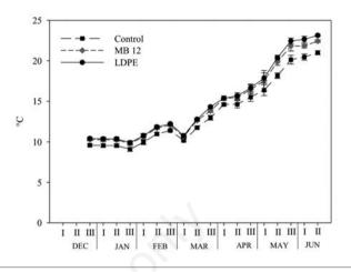
Figure 2. The trend of mean soil temperature under mulching treatments (bare soil, Control; soil covered by the black biodegradable film, MB12; soil covered by commercial black low-density polyethylene, LDPE) during the two crop cycles.
