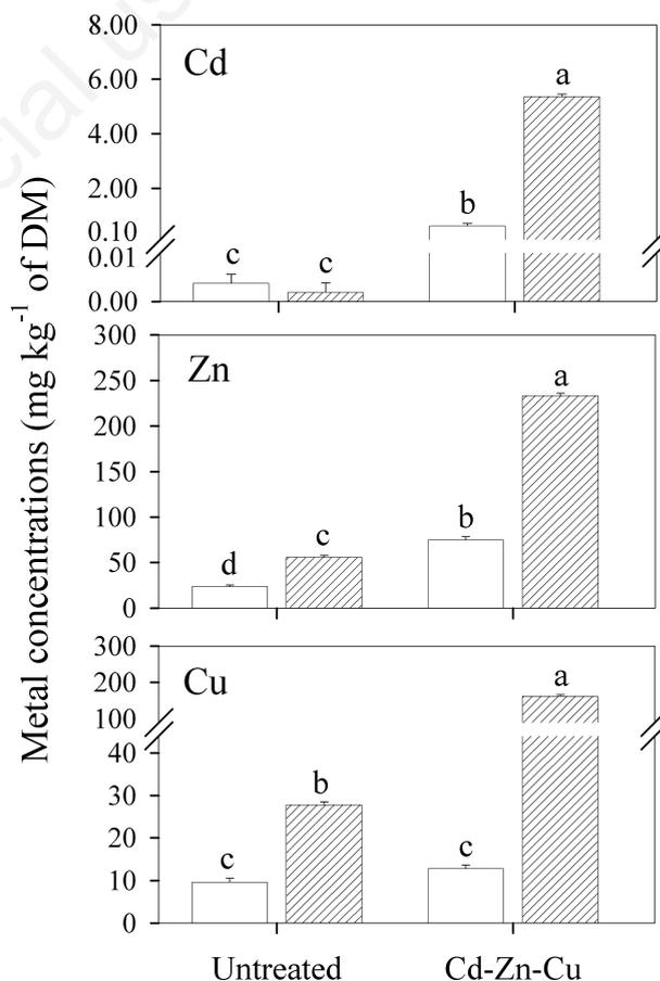
Figure 2. Metal concentrations in the aerial part (white bars) and roots (pattern bars) of sunflower at the flower bud stage. Values are means ( $n=4$ )  $\pm$  SE. For each metal, bars followed by the same letters are not significantly different for  $P \leq 0.05$  according to Duncan's test. DM, dry matter. Cd, cadmium; Zn, zinc; Cu, copper.
