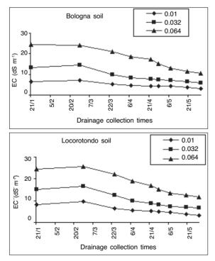
Figure 1. Evolution of drainage water electrical conductivity in the two soils during barley growing season, as related to the salt concentration of the irrigation water used in the previous four years (1999-2002).
