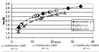
Figure 17. Relation between the hydraulic flow (Q) and log of saturated hydraulic conductivity (Ks).
