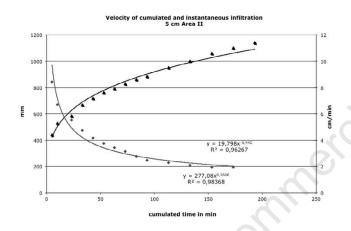
Figure 12. Cumulated and instantaneous hydraulic conductivity of Area II.
